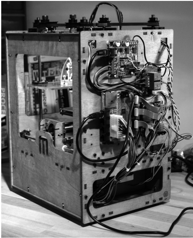
Figure 1-5. MakerBot CupCake 3D printer with Arduino-compatible electronics
